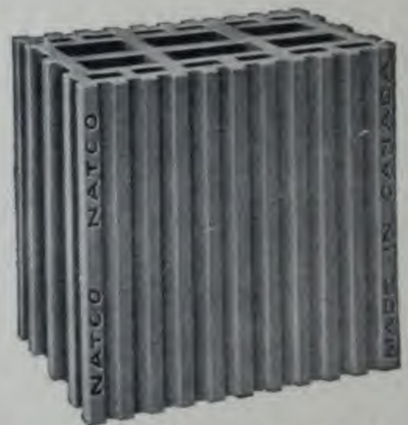
8" NATCO Double Shell Wall Tile Unit Showing dovetail method for gripping stucco on exterior and plaster on interior.
